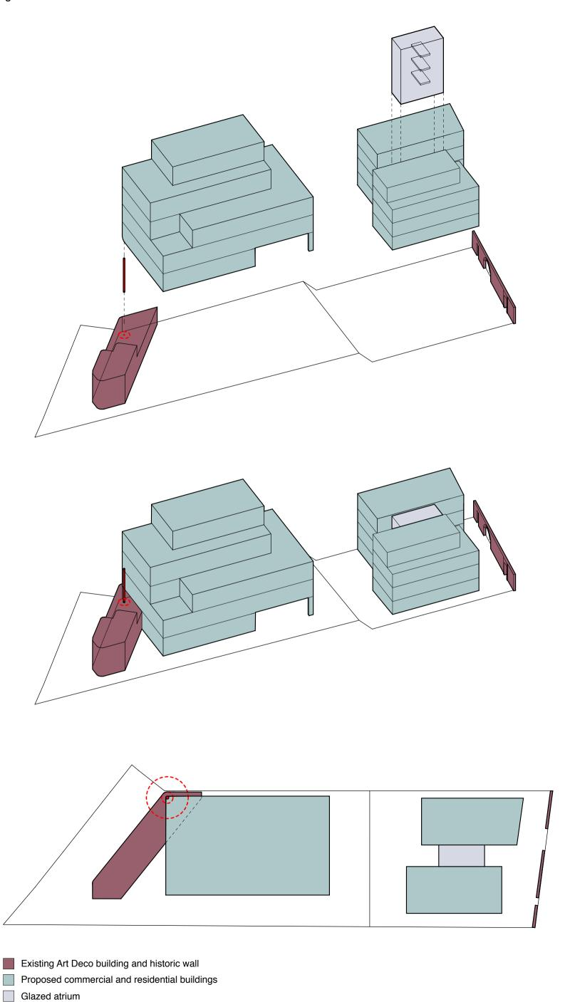
Existing geometry and setting out for new commercial building
